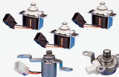
MS AXODE '97 FITS AXODE, '91-UP CONTINENTAL '92-UP TAURUS AND SABLE. WARNING: IF A .98 TO 1.6 OHMS ('92- '97) RESISTANT SOLENOID IS USED ON A SYSTEM REQUIRING A 13 TO 24 OHMS, ('98-UP) THIS WILL CODE YOUR COMPUTER. DO NOT INTERCHANGE MCCC SOLENOID! (LATE REQUIRES WHITE PLUG)
