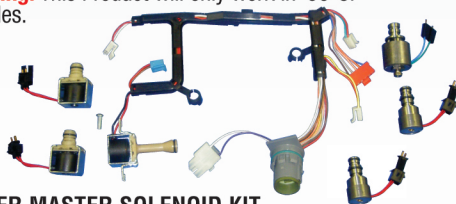
SUPER MASTER SOLENOID KIT MS 4L60E H Fits 4L60E '93-'95 With Solenoids and Internal Wiring Harness. Warning: will not work in '96-Up Vehicles.
