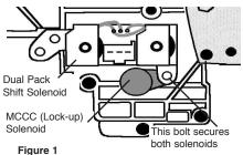
solenoid and the MCCC (Lock-up). Pull the dual solenoid directly out and discard. Remove the
