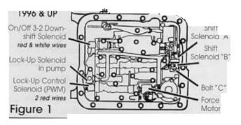
**2. To Install:** It is suggested that Bolt "C" be replaced with the torx bolt from the Kit to avoid a possible clearance problem
