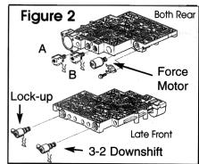
place. The force motor solenoid is installed with a retaining clip and a 10mm bolt. The PWM is the most difficult to install, because it is held in place with a U-clip that must be inserted from below into a journal in the valve body. Tighten all bolts according to normal OEM specifications. Both **A** and **B** shift
