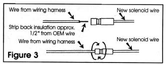
Tighten the connector. Repeat this procedure for all of the connections (Figure 3).
