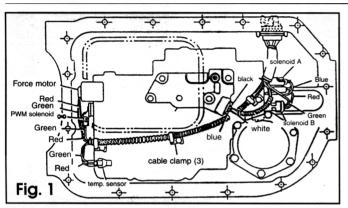
**1. To Remove:** Unplug the solenoids. Label each pair of wires on the harness so as to not confuse them. Remove the transmission filter, exposing the clip and the bolt on the force motor solenoid and the U-shaped retaining clip for the PWM solenoid. **Do not cut the PWM and Shift connectors.** Cut the wire connectors to the force motor solenoid as close as possible to the connector. Remove the force motor solenoid
