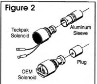
4. To Install: Install the aluminum sleeve furnished in the kit (Figure 2).
