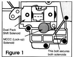
both the dual solenoid and the MCCC (Lock-up), Pull the dual solenoid directly out and discard. Remove the MCCC Lock-up Solenoid.
