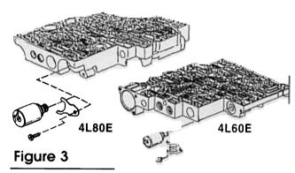
**5.** Test drive the vehicle to perform shift test. After driving the vehicle, it may be necessary to make the shift firmer or softer. To accomplish this, adjust the force motor solenoid. You will need a 3/8" and 5/8" wrench.
