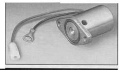
NOTE: This solenoid is used only in the DCC position on '93 Mitsubishi, and later Hyundai and Chrysler vehicles with a 13 ohm resistance. It will work for KM-175, 176 and 177 Series transmissions. IF A 3 OHM RESISTANCE SOLENOID IS USED ON A SYSTEM REQUIRING A 13 OHM SOLENOID, THE COMPUTER WILL BE DAMAGED. There are two methods to determine which ohms of resistance DCC (Lock-up) Solenoid is needed.
