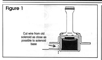
1. To Remove the old solenoid from the transmission, cut the wires from the old solenoid as close as possible to the metal base (Figure 1).
