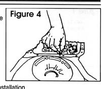
Caution: The K77929U Solenoid contains a diode. Polarity must be observed.
