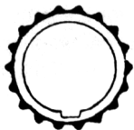
Figure A Typical 18-tooth gear. Count lobes from end of gear.
