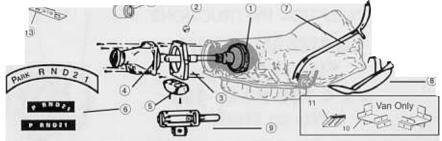
1. Install output shaft (Item #1) in the 400 transmission.
