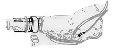
1. Select a 350 non lock-up transmission with a 9" extension housing.
