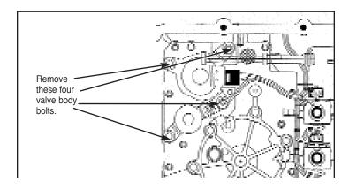
Use this solenoid as replacement in only those models originally equipped with OEM solenoids having a blue connector If in doubt, it is advisable to check the resistance of the solenoid being replaced. **1. To Remove** the old MCCC Lock-up solenoid, unplug the harness from the old solenoids, and remove the four 8mm bolts holding the EPC and MCCC Lock-up solenoids to the valve body (**Figure 1**). Remove the EPC solenoid. Remove MCCC Lock-up solenoid.
