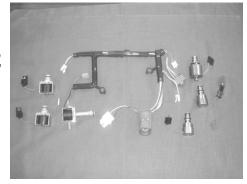
IMPORTANT: The only difference between 4L60E & 4L60E '96 early and late Master Kits is the 3-2 downshift control solenoid. Early is 9-14 ohms (two red wires). Late is 20-31 ohms (red and white wires).
