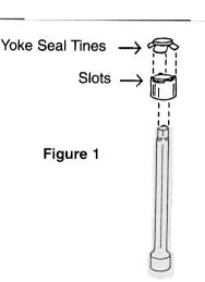
The tool will guide the yoke seal straight down the yoke.
